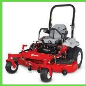
60 inch or 72 inch ride on mower. Used in larger open spaces, best in dry conditions.
